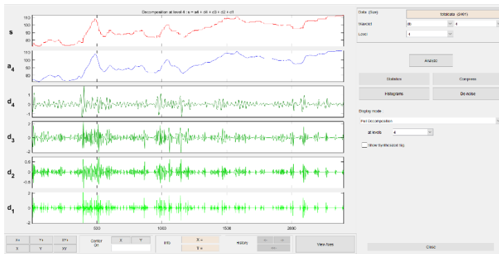
Figure 9. HR signal of the first subject in the wavelet domain in the state of physical stress.
