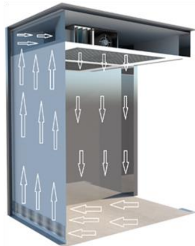
Figure 3. Illustration of the air circulation, purification, and disinfection process in the elevator cabin.
