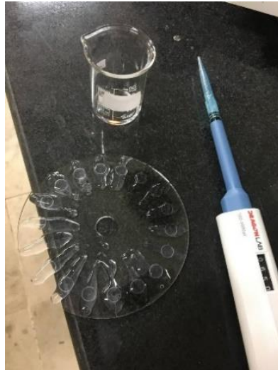
Figure 5. A representation of the equipment required for coating the PMMA chip with a solution of water and agarose nanoparticles to enhance hydrophilicity.
