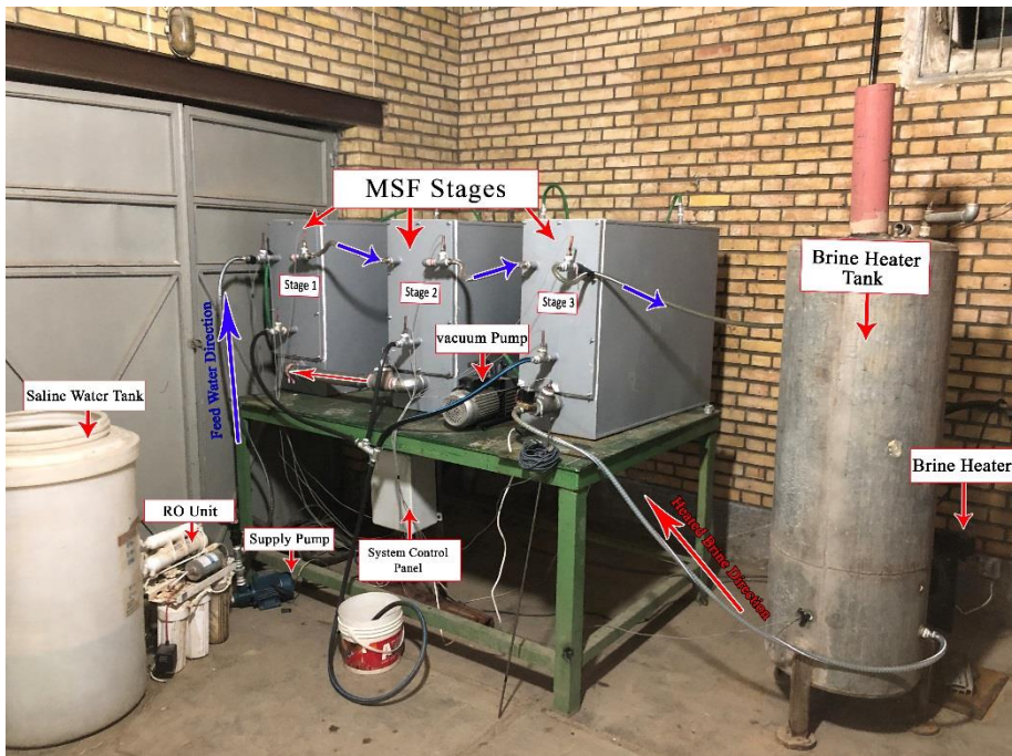
Figure 1. Desalination System Unit.
