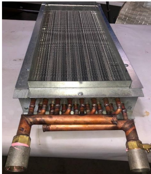
Figure 5. Condenser of the Desalination System Unit.
