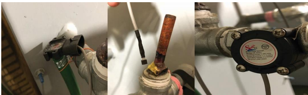
Figure 7. Pressure Sensor, Temperature Sensor and Flow Meter of the Experimental System.
