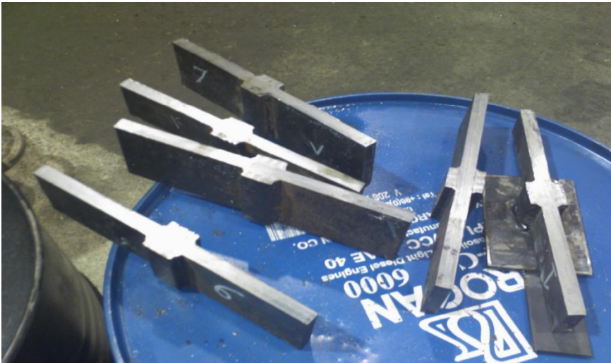
Figure 4. Cutting of the sample for mechanical tests.
