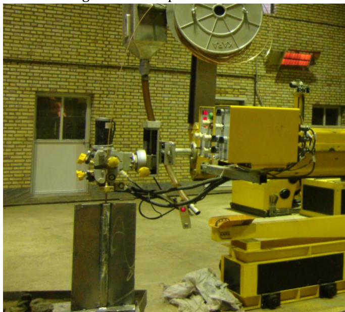
Figure 3. Way the part is placed for welding.
