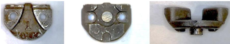
Figure 3. Different views of the manufactured part using MIM
