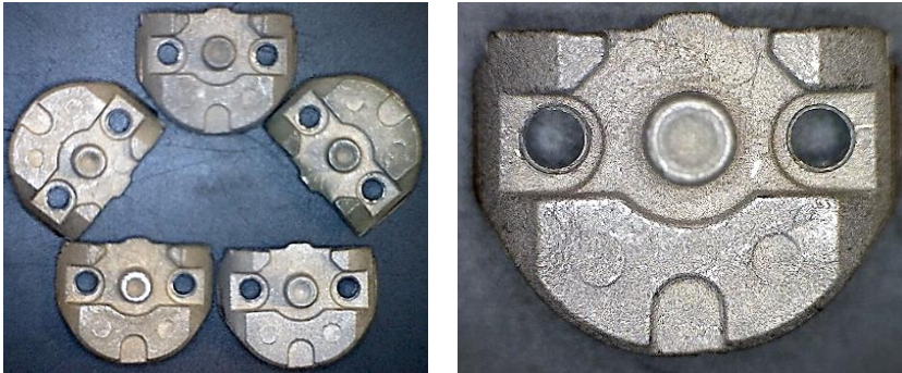
Figure 6. Manufactured samples processed with protective argon gas.
