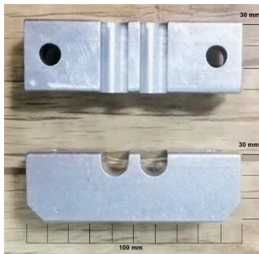
Figure 2. A sample of manufactured aluminum alloy 6061-T6 part
