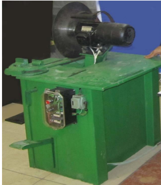
Figure 10. Fire saw industrial cutting machine equipped with intelligent system
