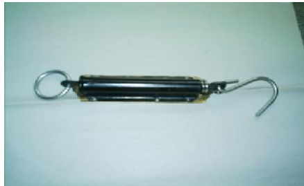
Figure 2. Force gauge to measure the static force to separate fruit
