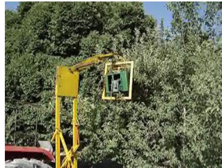
Figure 8. Vibration mechanism for transfer vibration to stem
