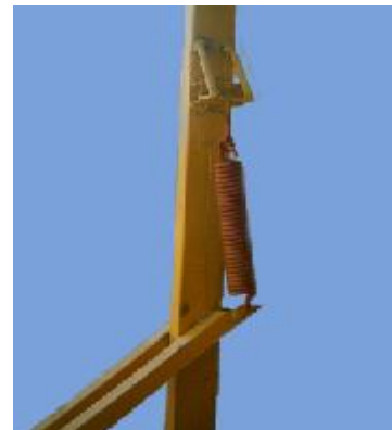
Figure 8. Vibration mechanism for transfer vibration to stem
